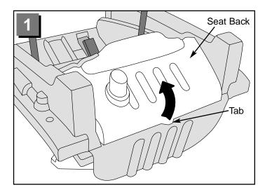
Lift the tab on the back of the seat back to unlatch the peg from the hole in the vehicle body.
